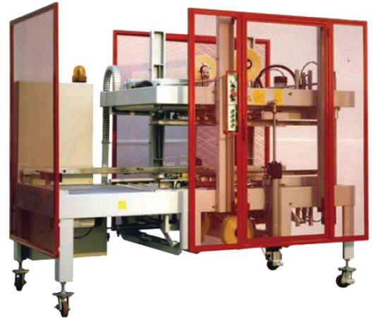
Above unit shown is right side infeed. Front infeed protection on the left is an available option at additional cost.
